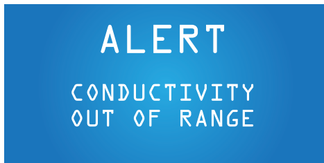
#4 PRIORITY Alert Conductivity This message appears when the aquarium water conductivity is outside the set range. For further instructions visit www.fluval-g.com .
