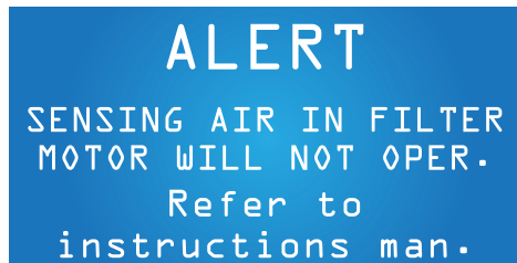
#1 FIRST PRIORITY Sensing air in filter This message appears when there is not enough water in the filter. For further instructions visit www.fluval-g.com .
