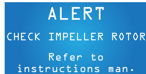
#2 PRIORITY Blocked Impeller This message appears when the impeller is blocked and the filter is not pumping water. For further instructions visit www.fluval-g.com .
