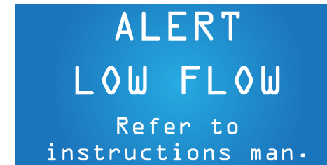
#5 PRIORITY Low Flow This message appears when the water flow is equal or below the factory-set minimum. For further instructions visit www.fluval-g.com .
